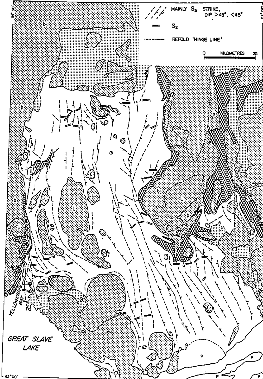
Figure 4.2 S_2 and S_3 fabrics and refold hinges of the Yellowknife Basin taken from Fyson (1984b, Figure 3). Rocks type patterns similar to Figure 4.1.
